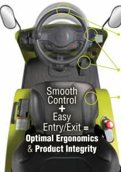
26° Tilt Steering Column maximizes operator's driving preferences.
